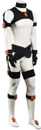
Figure 2. The belts/straps system of Xsens, equipped with MEMS
