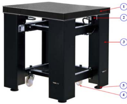
Figure 6. Subsystem of the anti-vibration table: 1- breadboard, 2- self-leveling mechanism, 3- mechanical frame, 4- rollers for travel, 5- adjustable support
