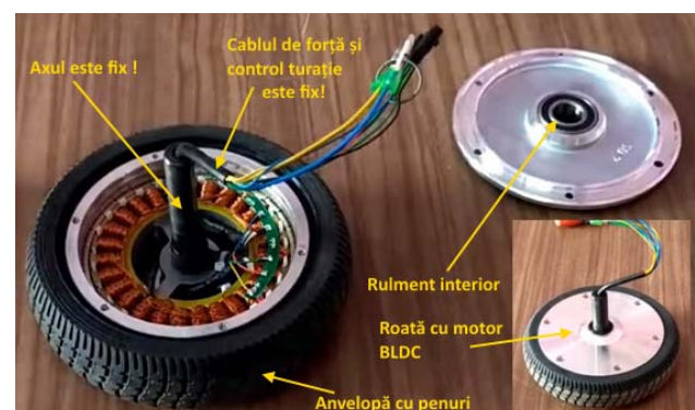
Figure 1. Brushless three-phase BLDC motor, integrated inside the wheel, a cutting-edge novelty in mechatronics
