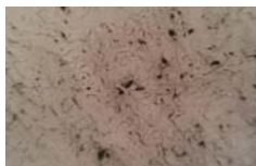
Figure 1. Microstructural appearance on an unetched sample. Perlite, max. 5% ferrite and lamellar graphite with graphite lamellae length 4 -5 (batch 1) Magnification x100
