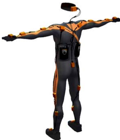
Figure 3. The Lycra-type bodysuit of Xsens, equipped with MEMS
