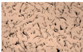
Figure 3. Microstructural appearance on an unetched sample. Perlite structure, max. 5% ferrite and lamellar graphite with graphite blade length 4 (batch 2) Magnification x100
