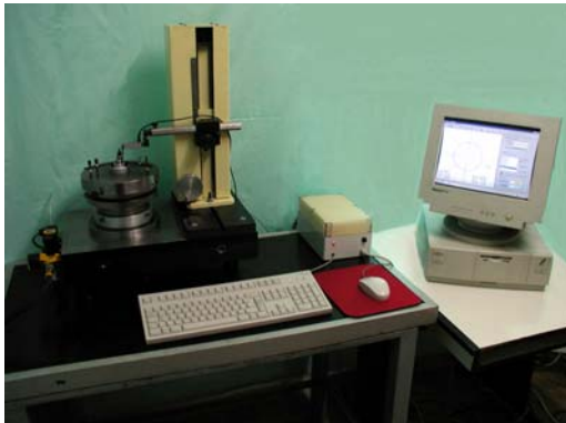
Figure 10. Device for measuring shape deviations of circular parts also using data processing methods based on Fourier transform
