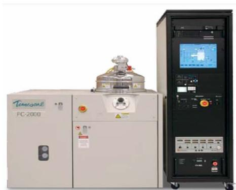
Fig. 1: TEMESCAL FC-2000 –deposition system by electron beam evaporation
