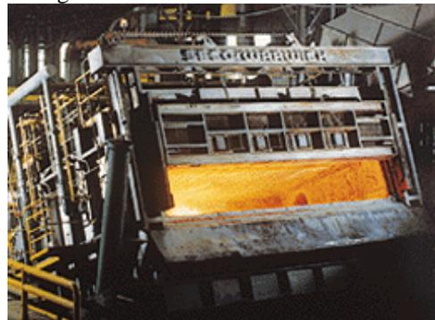
**Fig.2 View from the swing filling door of an aluminum melting furnace**
