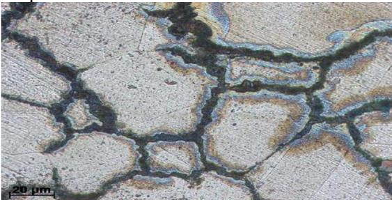
**Fig.9 The sample microstructure of the heat affected zone with a length of L=25mm (x500)**
