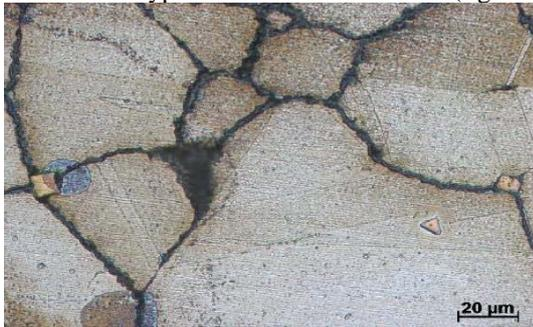
**Fig.8 The sample microstructure of the heat affected zone with a length of L=100mm (x500)**
