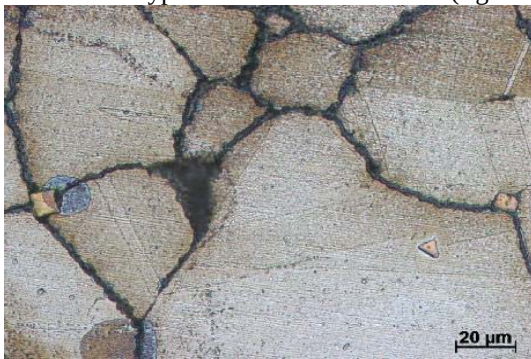
Fig.8 The sample microstructure of the heat affected zone with a length of L=100mm (x500)
