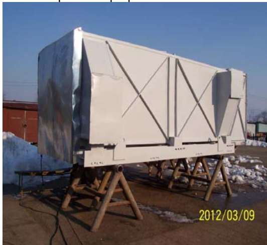
Fig.10 View of the repaired pre-heater from the flue gas entrance zone towards the tubesheet, covered by a metallic sheet for transportation purposes
