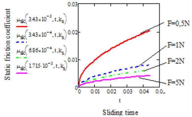
Fig. 2. Evolution of the static coefficient function on loading and parking time
