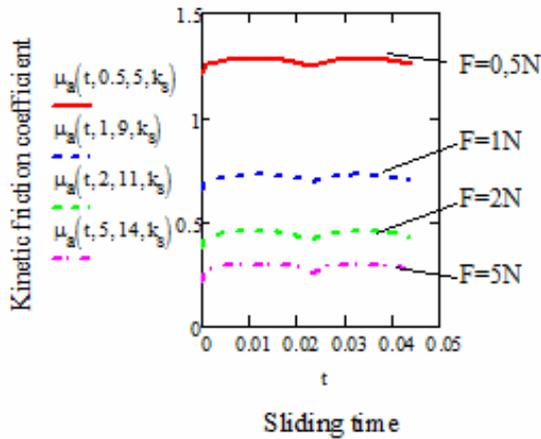
Fig. 1. The evolution of the kinetic friction coefficient function on the loading conditions and sliding time
