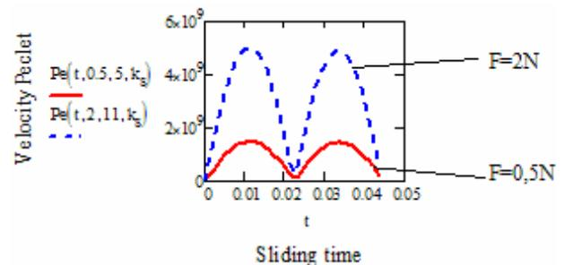
Figure 5. Dimensionless velocity variation during stick-slip sliding
