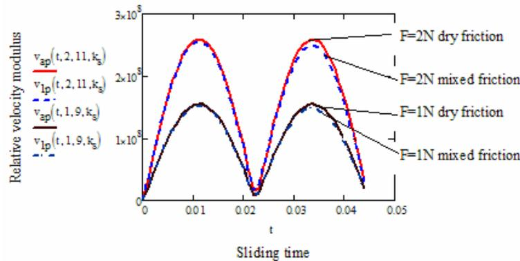
Fig. 4. Evolution of the relative velocity modulus during sliding in case of dry and mixed friction
