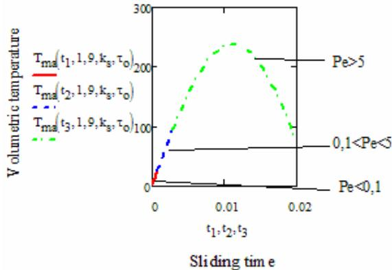
Fig. 6. Evolution of dimensionless volumetric temperature during sliding
