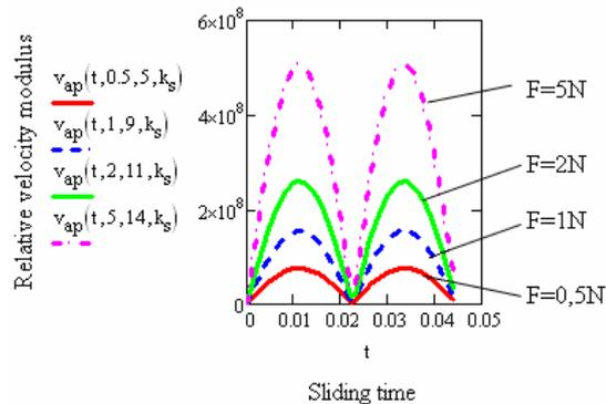
Fig. 3. Relative velocity modulus during sliding in case of dry friction
