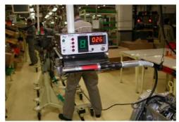
Fig. 14. Digital torque wrench for rocker-arms assemblage
