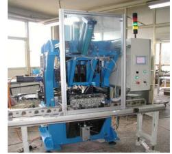
Fig. 11. Tappets controlling and sorting machine with dynamic mobile
