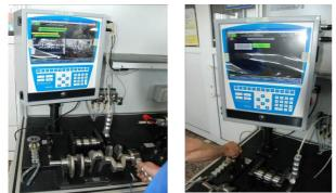
Fig. 9.Crankshafts control equipment H4x OP.200-210
