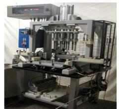
Fig. 16. Equipment for tightness control of cylinder head and marking
