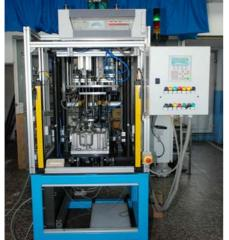
Fig. 17. Intelligent mechatronic equipment for measuring the tightness of the cylinder carter assembly
