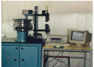
Fig. 5. Installation equipped with computers for measuring radial and axial run out on rim
