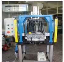
Fig. 19. Intelligent mechatronic technology and equipment of tightness control for assembled cylinder head of F8Q engine
