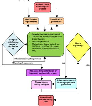
Fig. 3. Process design and execution of mechatronic systems
