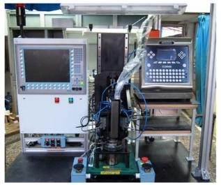
Fig. 6. Mechatronic equipment for geometric control and marking of drum parts
