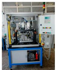
Fig. 15. Tightness control intelligent mechatronic equipment (in vacuum) for gear carter JH3
