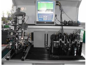
Fig. 8. Mechatronic control equipment for crankshafts
