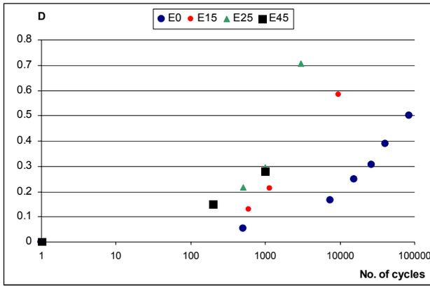
**Figure 5. The evolution of composite degradation with number of cycles**
