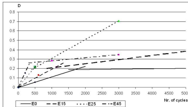
**Figure 6. Highlighting the two stages of bending fatigue damage in hand made stratified composites**
