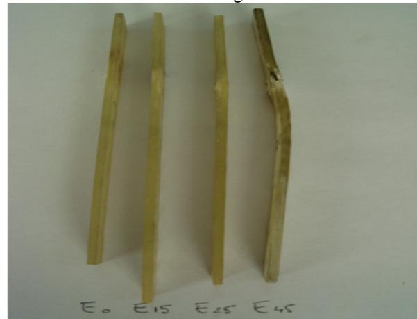
Figure 8. Specimens appearance after bending fatigue loading
