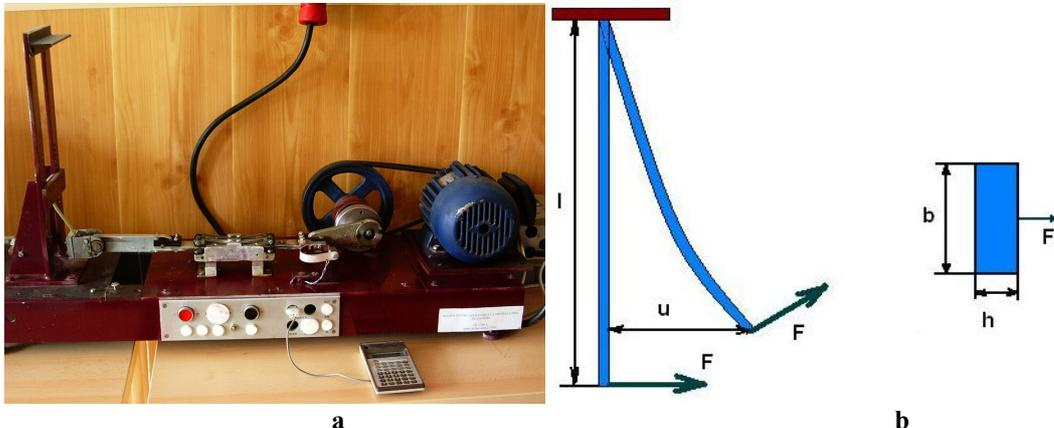
Figure 1. Overview of bending fatigue testing machine (a) respectively, specimen geometry and loading mode during fatigue tests (b)
