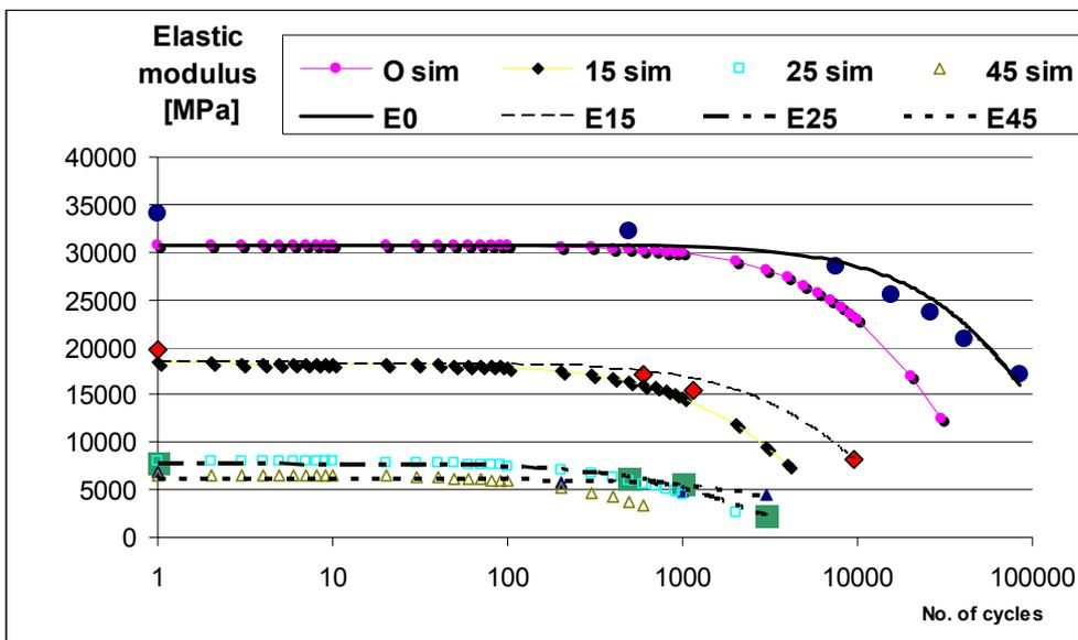
**Figure 4. Comparison between experimental curves and model with calculated parameter  $m$**
