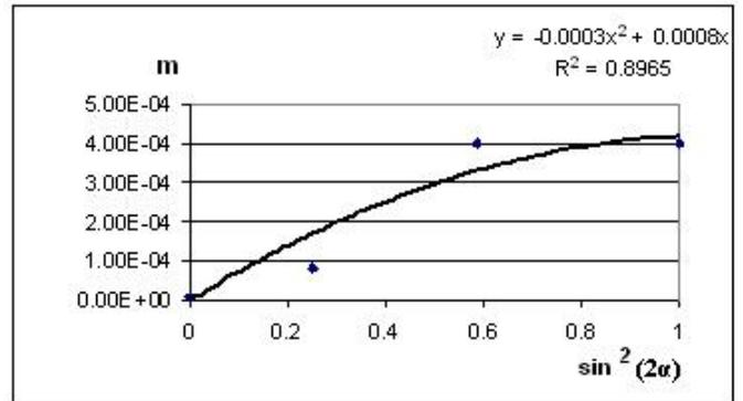
**Figure 3. Exponent value  $m$  from equation (2) as function of angle between the cut out direction of specimen and reinforcement direction**
