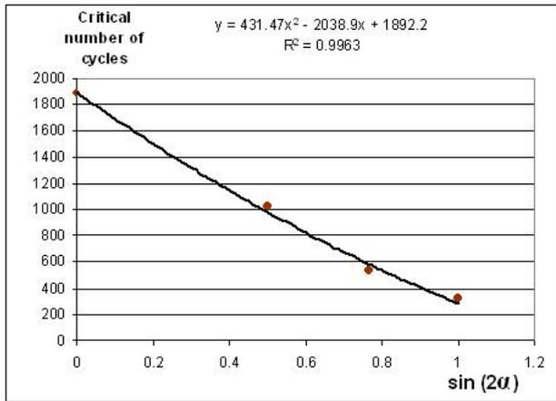
Figure 7. Correlation between the critical number of cycles and the direction of cut out specimens
